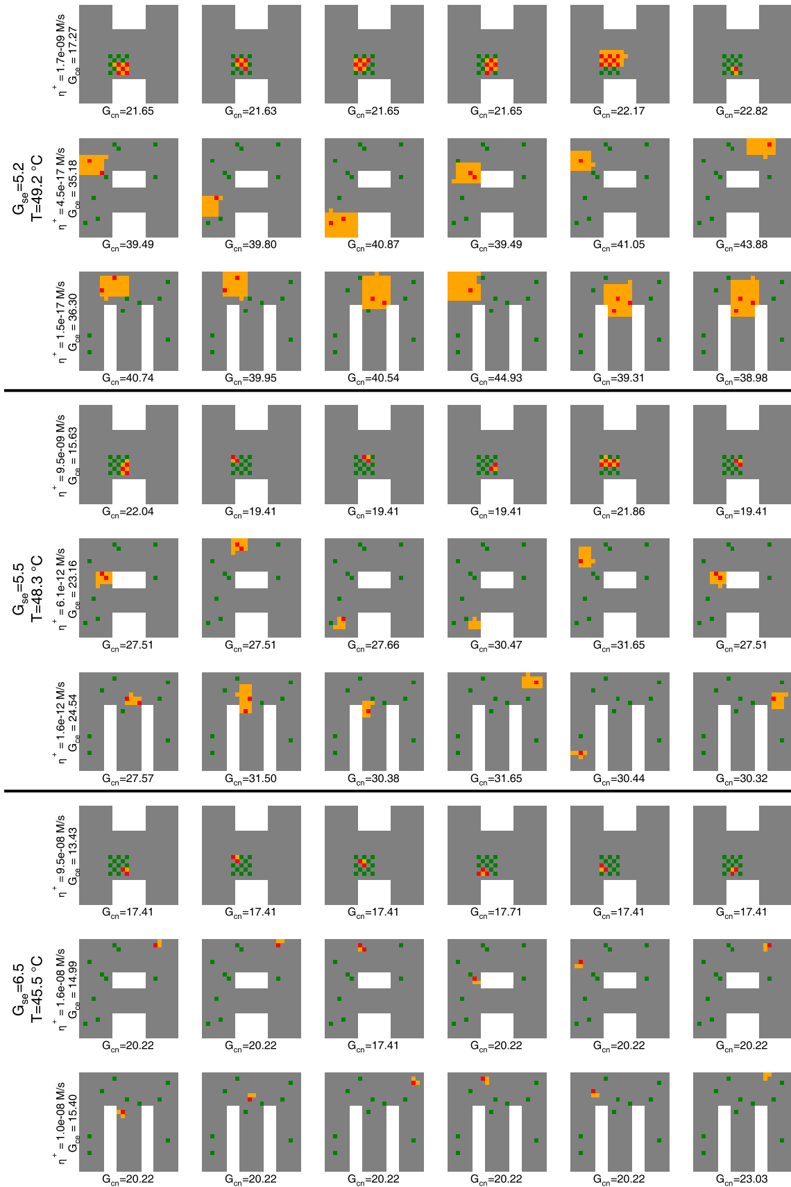
Figure 1.1: A Boltzmann-weighted sample of 6 'critical nuclei' for each shape, at three temperatures, for H flag 6. Orange and red indicate low- and high-concentration tiles that are part of the critical nucleus, respectively; grey and green are used analogously for tiles not in the nucleus. \eta^+ is the estimated nucleation rate for the shape; G_{se} is the corresponding critical nucleus ensemble free energy; G_{se} is per-bond differential sticky-end energy at the shown temperature; and G_{en} is the chemical potential of the given critical nucleus.
