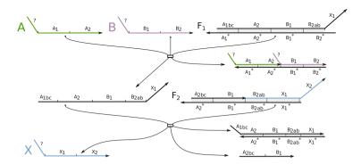
**Fig. 4.** An implementation of X := AND(A, B) using the DLD motif and cooperative hybridization.
