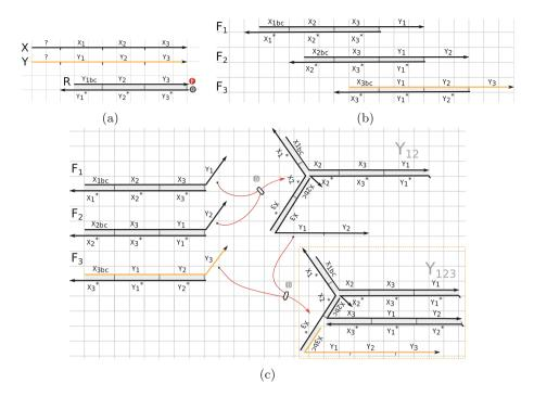
**Fig. 6.** An implementation of the translator Y := X that uses the triple long domain (TLD) motif. (For simplicity, we show this scheme without clamps.) (a) Input signal and output signal format, and downstream reporter complex, R. (b) Fuel complexes. (c) A coarse grained leak pathway showing only bimolecular reactions.
