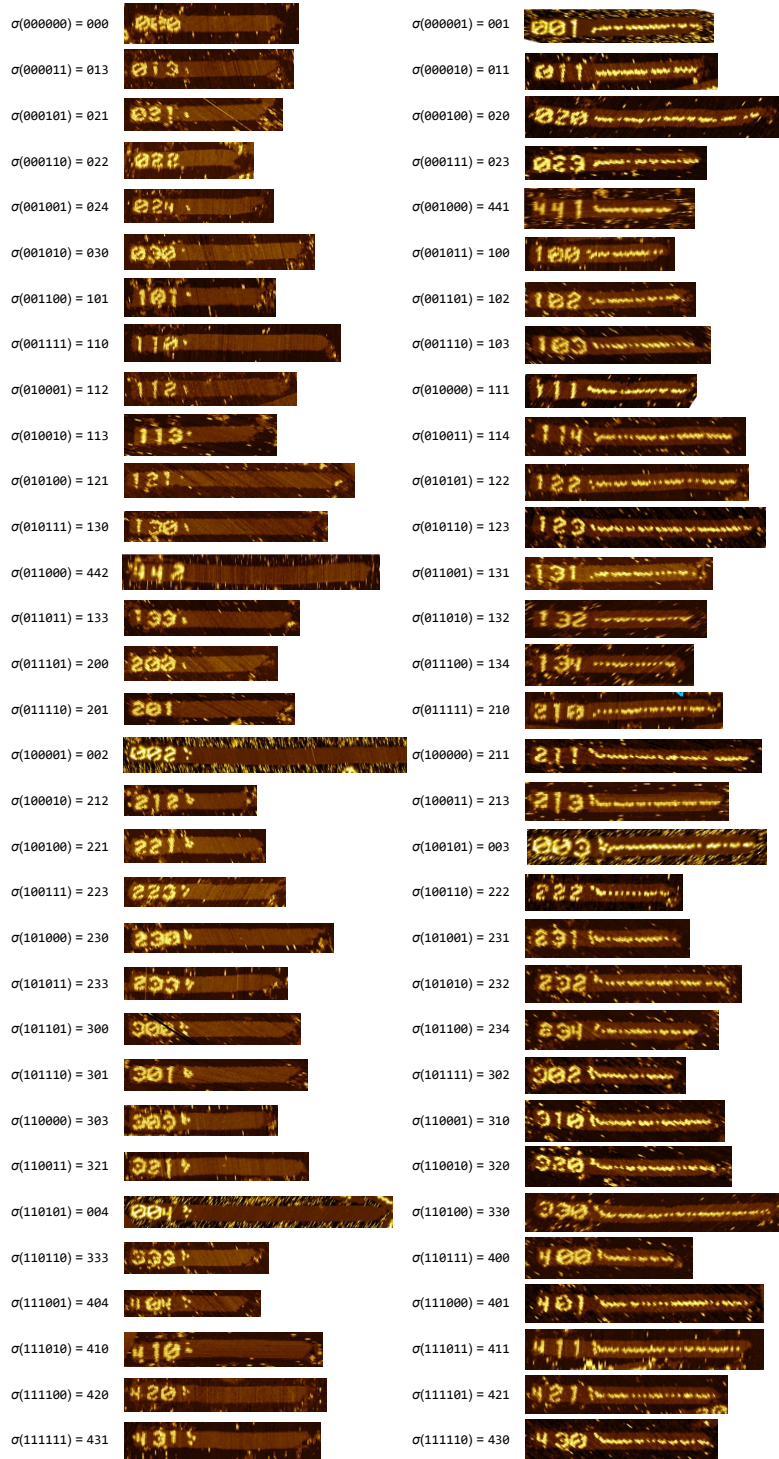
Figure S44: PARITY circuit on all 64 inputs, showing one nanotube for each input. ‘No’ instances of the parity problem are on the left, ‘yes’ instances are on the right. The notation \sigma(x_0) can be read as: “The seed label for input bit string x_0 ”.
