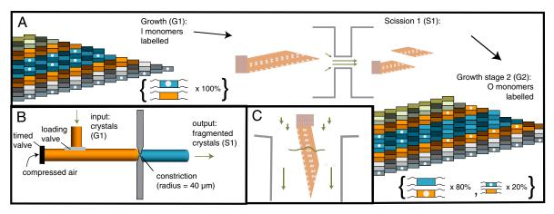
Fig. 2. Replication stages. (A) After growth (G1), crystals undergo scission (S1) and further growth (G2). (B–C) Scission mechanism. Compressed air propels solution containing crystals through a constriction (B), where high elongational flows fragment crystals [zoom, (C)]. Arrow lengths indicate rough fluid velocity.
