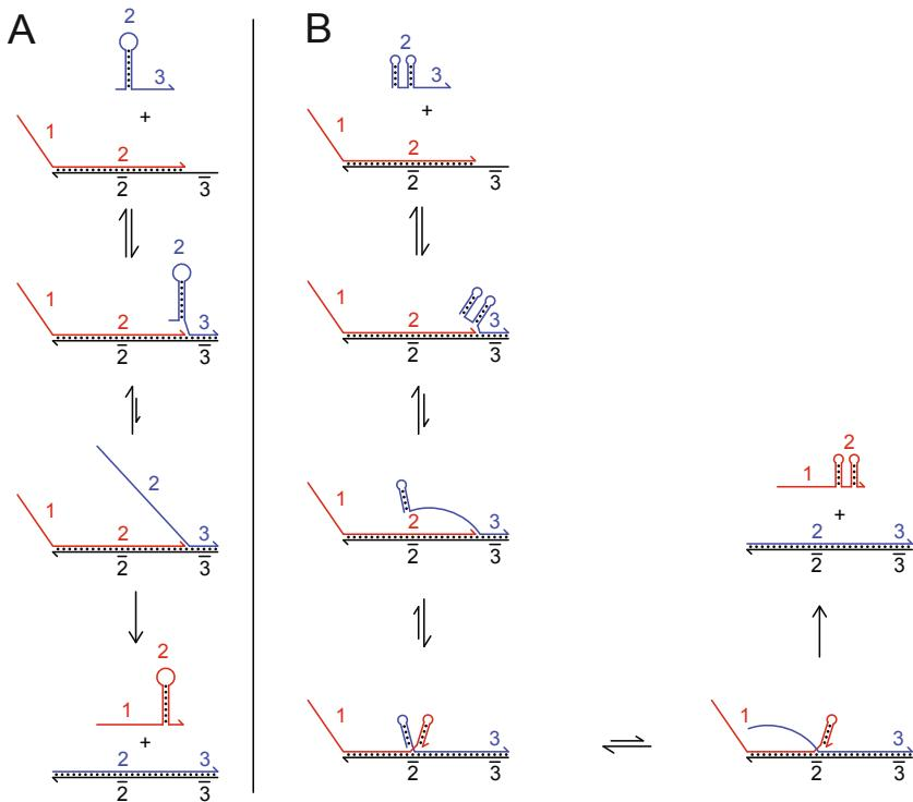
**Fig. 2.** Failure of thermodynamics-based sequence design. The  $\Delta G^\circ$  (standard free energy) of the folded domain 2 is more negative in (B) than in (A), but the sequential nature of branch migration means that the strand displacement reaction involving (B) could be faster than that of (A).
